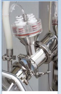
+ The test tablet dispenser KT2010 is an innovation that allows for easy contained metal detector sample tablet insertion without breaking containment
